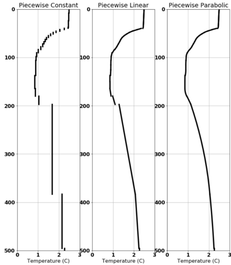
Fig. 3: Polynomial reconstructions, starting with piecewise constant on the left, piecewise linear in the middle and piecewise parabolic on the right.
